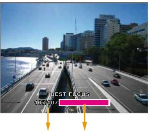
The color bar fluctuates according to current focus value.
